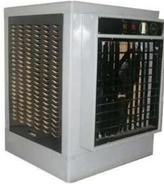
An exhaust fan is mounted inside a cooler housing and vertical sides of the cooler housing are fitted with cooling pad. These pads are kept wet with the help of water pump. Rotation of fan mounted inside the body draws air from all the three sides through wet pads. Thus, air gets cooled by evaporation of water and which is blown into the room. Air coolers have advantages such as, they are easy to maintain, budget friendly, and portable, compared to air conditioners. Types of air coolers are -
